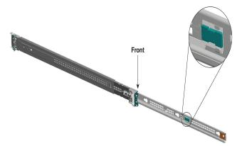
Slide the plastic tab forward, and pull the inner slide rail to disconnect it from the outer slide rail.
